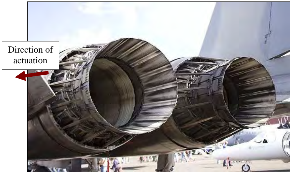
Figure 2.7.2 Linear actuators placed parallel to flow on the F-15 Eagle Fighter. The actuators tug directly along the nozzle. (Source: UAV News)
