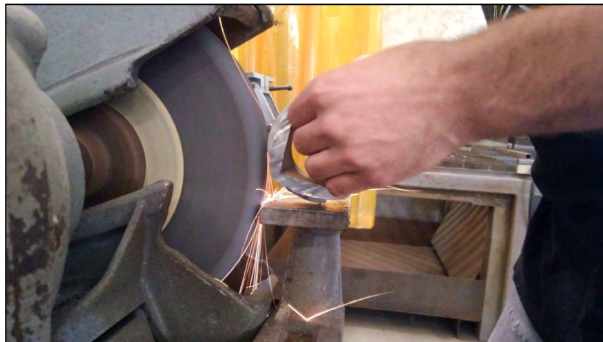
Figure 7.5.1 Grinding the Sides of a Stainless-Steel Part
