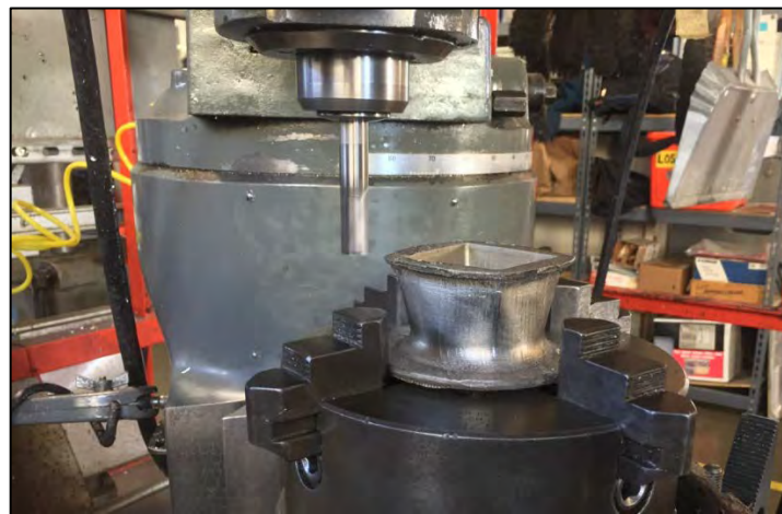
Figure 7.2.2 Face Milling Top Surface of Throat
