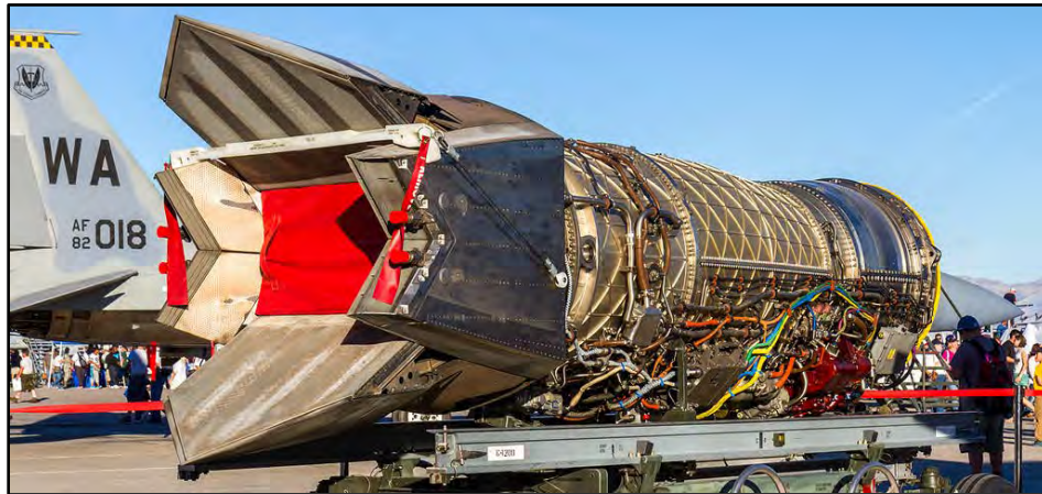
Figure 2.5.1 The F119-PW-100 engine and nozzle. Both sides are flat fixed flaps, while the top and bottom sides are curved plates that are independently actuated, allowing vectoring as well as converging and diverging. (Source: John Pike)
