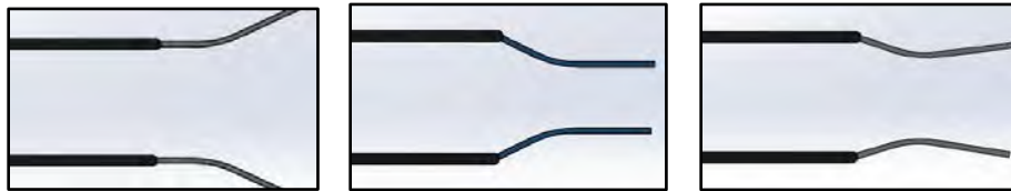
Figure 4.3.4 The three positions of the curved-flap rectangular nozzle allows for pure-diverging (left), pure converging (middle), or converging-diverging (right) nozzle shapes.
