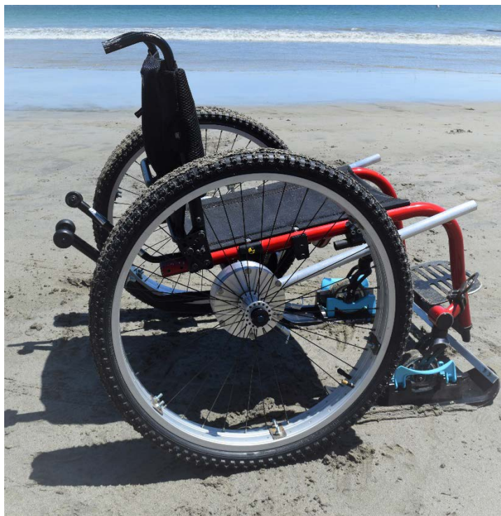
Figure 32. Final design on the beach. The wheelchair was tested and proven that our beach wheelchair attachment worked effectively in sand.
