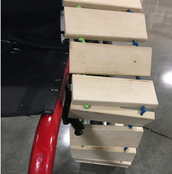
Figure 9b. Rope Ladder and TiLite wheelchair The rope ladder track attachment on the wheelchair.
