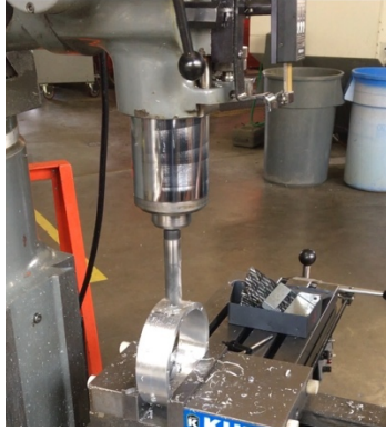
Figure 25. Outer sleeve on Mill The hole for the lever arm was drilled into the outer sleeve using a mill.
