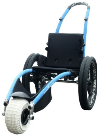
Figure 12. The Hippocampe wheelchair uses a dual wheel for the main wheels on each side. This has proven to work well in the sand.
