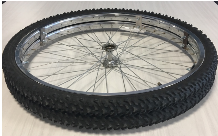
Figure 13. The Double Wheel Prototype. The prototype is two bike rims attached by metal brackets. One rim has spokes while the other doesn't.
