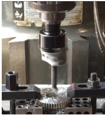
Figure 26. Boring Tool The inner diameter of our ratchets was increased using a boring tool on a mill.
