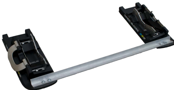
Figure 20. The Front Wheel Subassembly A crossbar was added to limit the amount of turning that the front wheels can experience.
