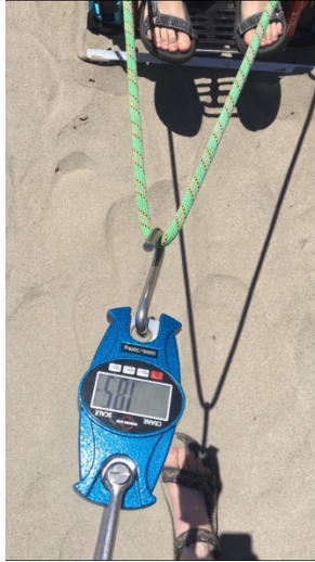
Figure 31. Force testing on soft sand. A crane scale was used to measure the force it takes to make one forward rotation.
