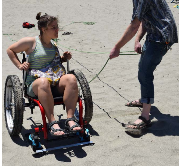
Figure 30. Distance Testing on Soft Sand. Rope was used to measure how far the chair moves after five strokes with the levers.
