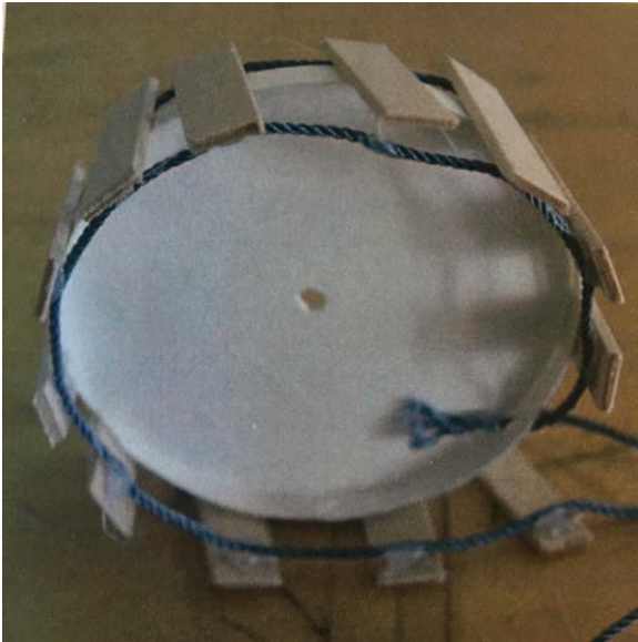
Figure 6. Rope Ladder Concept made of popsicle sticks were cut and attached with string to create a conceptual rope ladder track.
