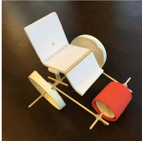
Figure 7. Roller Attachment Concept made from foam wrapped around a cylinder made of paper cups to show a roller mechanism in place of the two front wheels.
