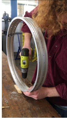
Figure 23. Double Wheel Manufacturing Holes are being drilled into the rims so that brackets can be used to attach the rims to one another.
