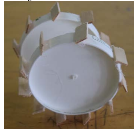
Figure 6. A treaded wheel was a simple design that we could modify in several different ways to get the prototype we wanted. The stress on the treads or 'scoops' would be too significant and hard to design for when prototyping.
