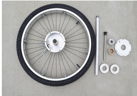
Figure 28. Assembled Double Wheels The double wheels are assembled with part of the hub assembled and the remaining parts to the right.
