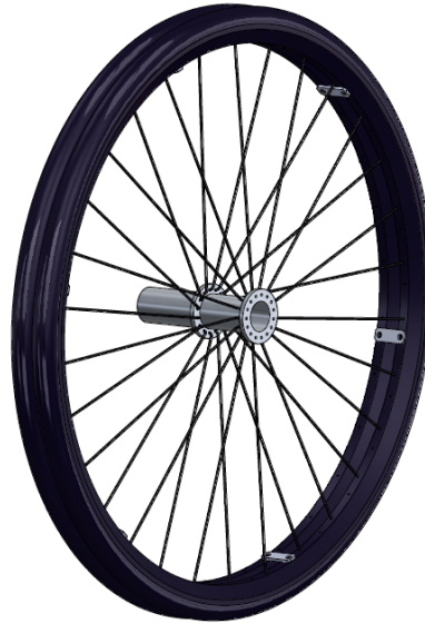
Figure 17. The Double Wheel Subassembly the wheelchair uses a dual wheel for the main wheels on each side. This has proven to work well in the sand and be user friendly.
