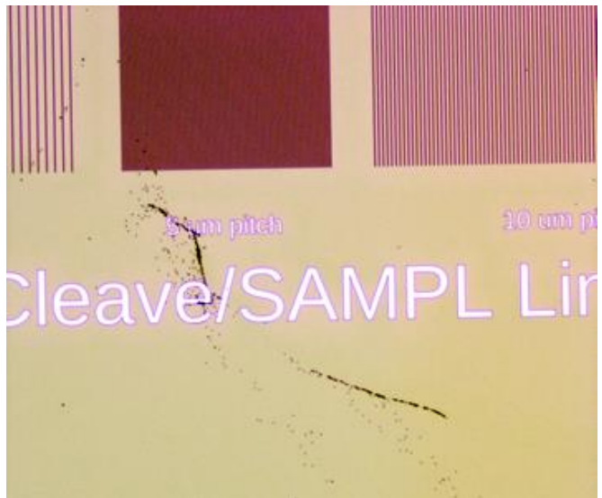
Figure 4: 2 μm pillar array deposited along the surface of the wafer
