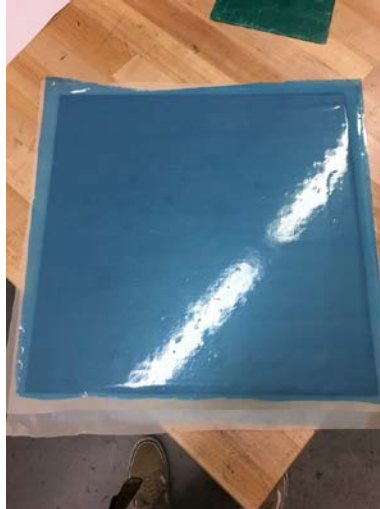
Figure 46. Carbon fiber seat plate setup before cure
