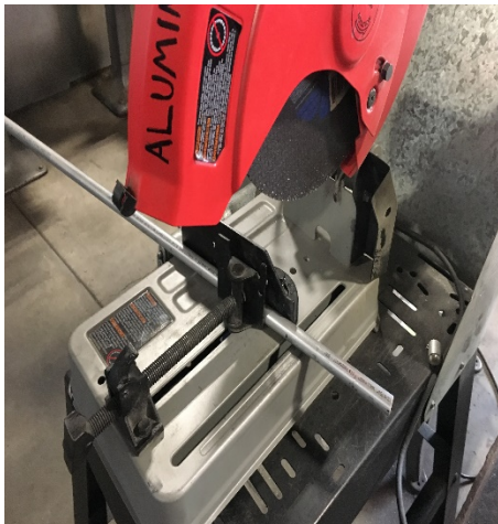
Figure 44. Backrest frame tubing being cut to length
