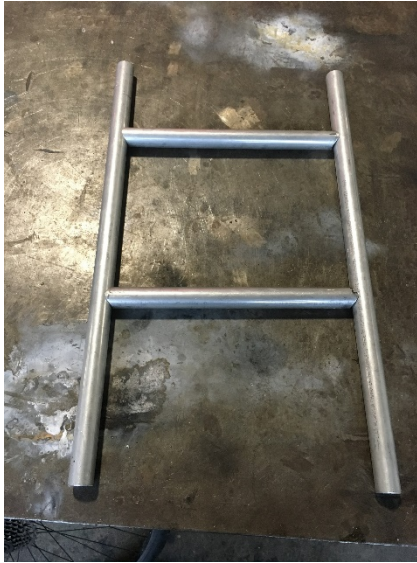
Figure 47. Tilt-in-space frame before welding
