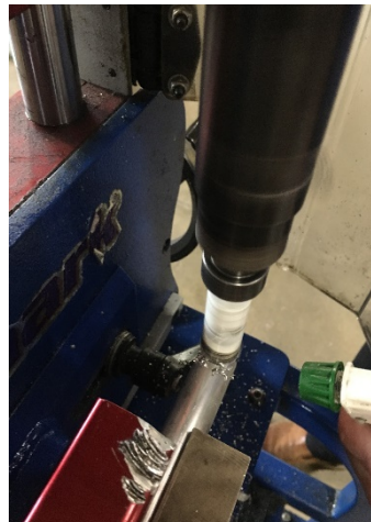
Figure 43. Backrest frame being notched
