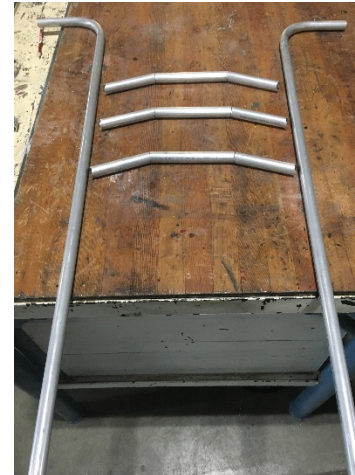
Figure 42. Backrest frame cut to length and shaped before welding
