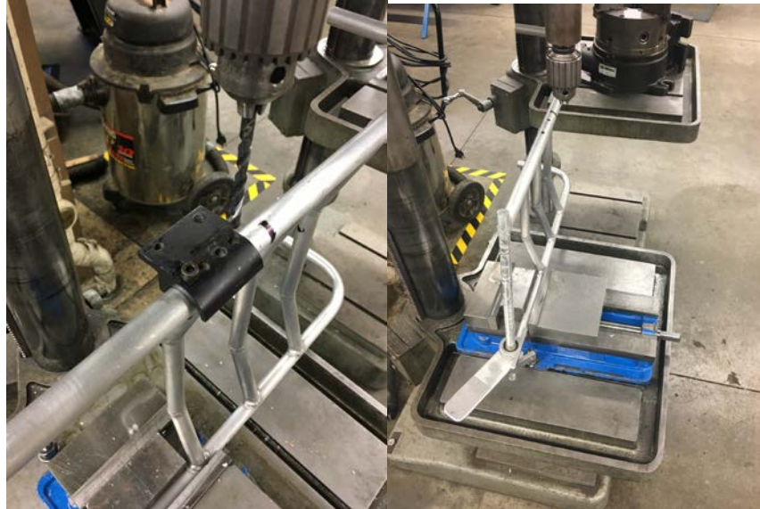
Figure 52. Backrest frame hole drilling to attach armrests
