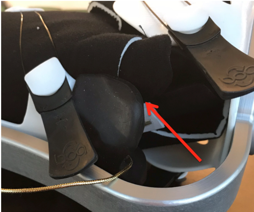
Figure 28. Pressure Sensor Placement during Preliminary Testing
