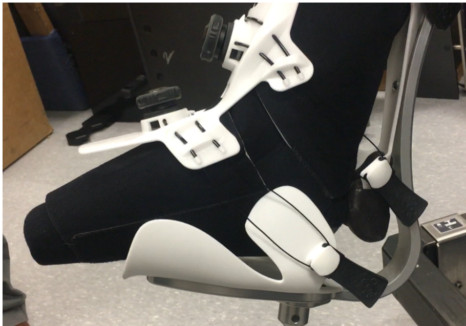
Figure 10. Stryker hip distraction boot after heel slip
