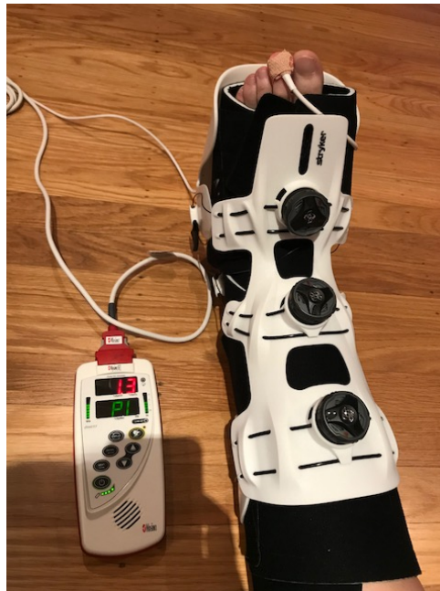
Figure 24. Masimo RAD-57 Test Setup with LNCS Neo-3 Adhesive Wrap
