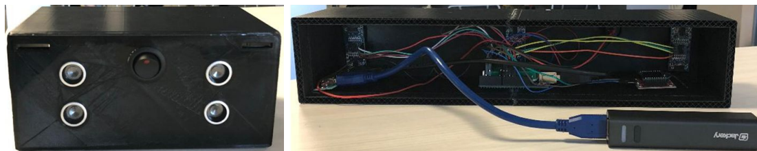
Figure 7.1.1.2 The front sensor housing (left) side sensor housing and side sensor housing (right) with full assembly of electronics.
