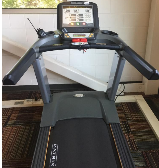
Figure 5.1.1. Larry's treadmill at his local YMCA. The greater arm lengths on this treadmill would allow for larger sensor mounting area.
