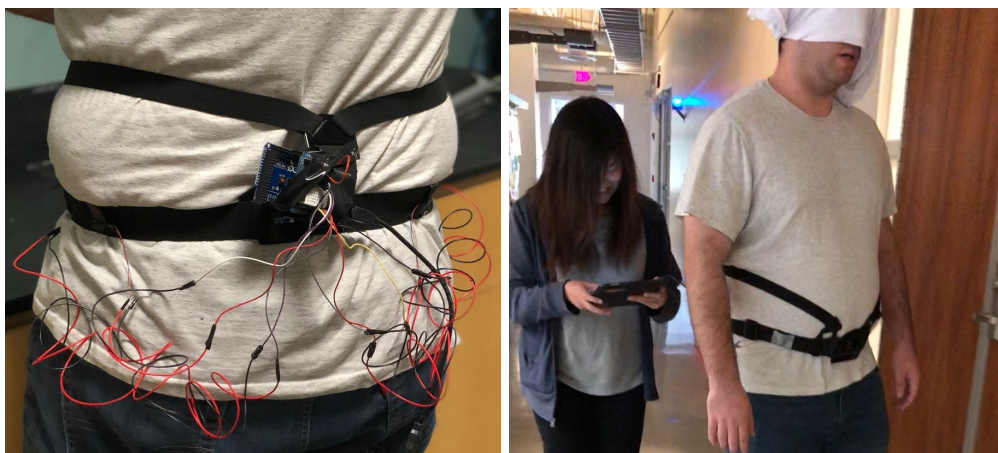
Figure 5.2.1 A GoPro harness with 4 coin motors and an Arduino Uno attached (left). A blindfolded motor code testing with a member of the team (right).
