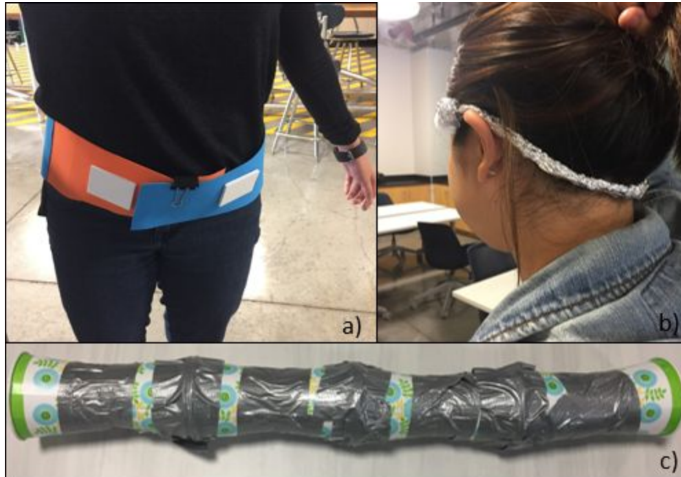
Figure 4.1.2. Feedback-providing concepts. a) Belt with vibrotactile motors. b) Sound feedback headband. c) Piping air feedback.
