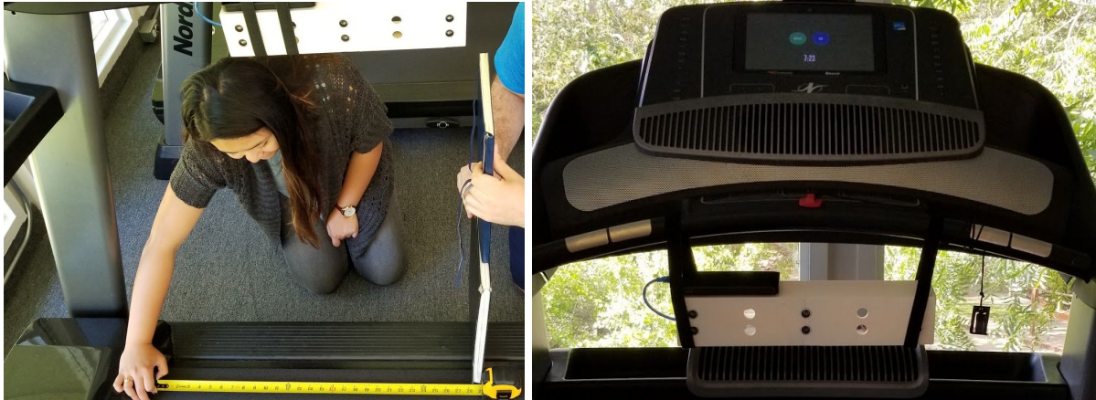
Figure 6.2.1.1. Measuring the placement of the right side sensor housing to cover the safe zone (left). New location of the front sensor housing after the first full system test (right).
