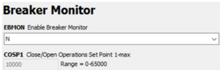
Figure B10: SEL-710 Breaker Monitor Settings
