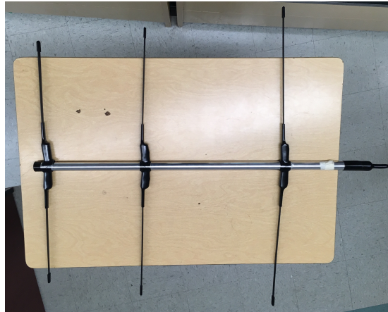
Fig. 6: Biotrack Yagi-Uda Antenna (from left to right: director, active element, reflector)
