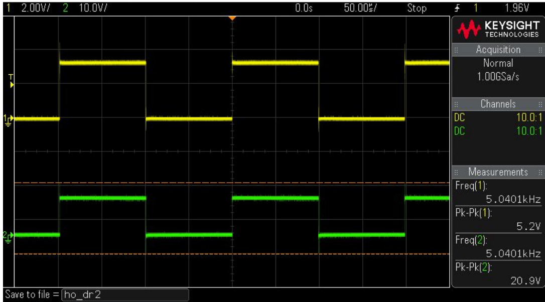
Figure 5-5: HI side Driver test with Function Generator Function Generator Input (Yellow) and Driver HI Output (Green)
