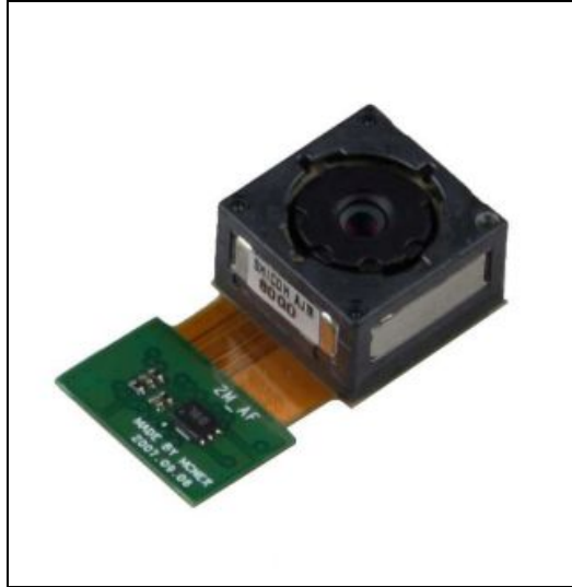
Figure 6: Micron MT9D111 camera module used for this project [5] .
