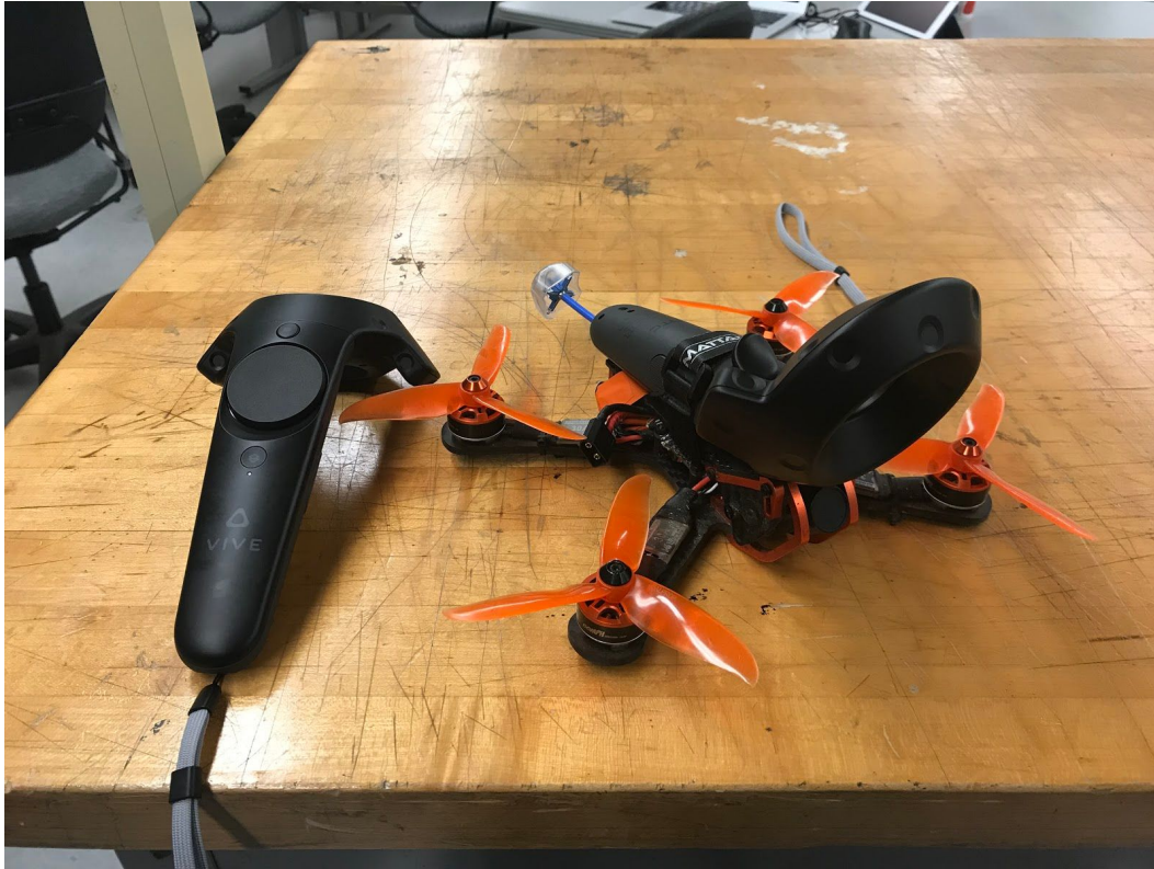
Figure 15 - Before the custom controller was built, the vive controllers were test mounted and flown with the program created “Valkyrie”
