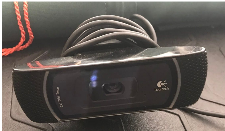
Figure 9 - Modified Webcam with IR filter removed
