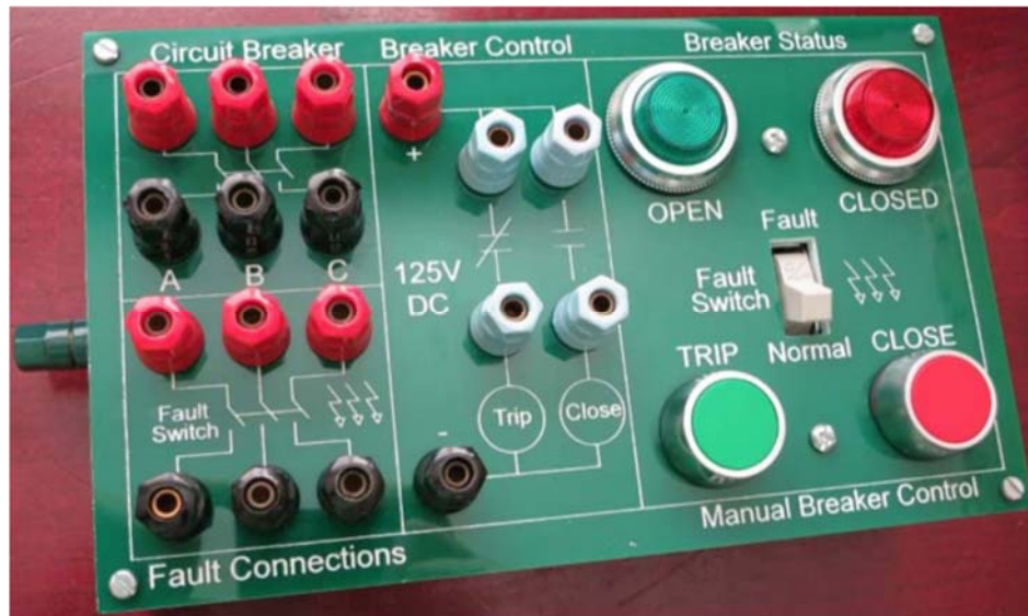
Figure 8: Circuit Breaker Front Panel [16]
