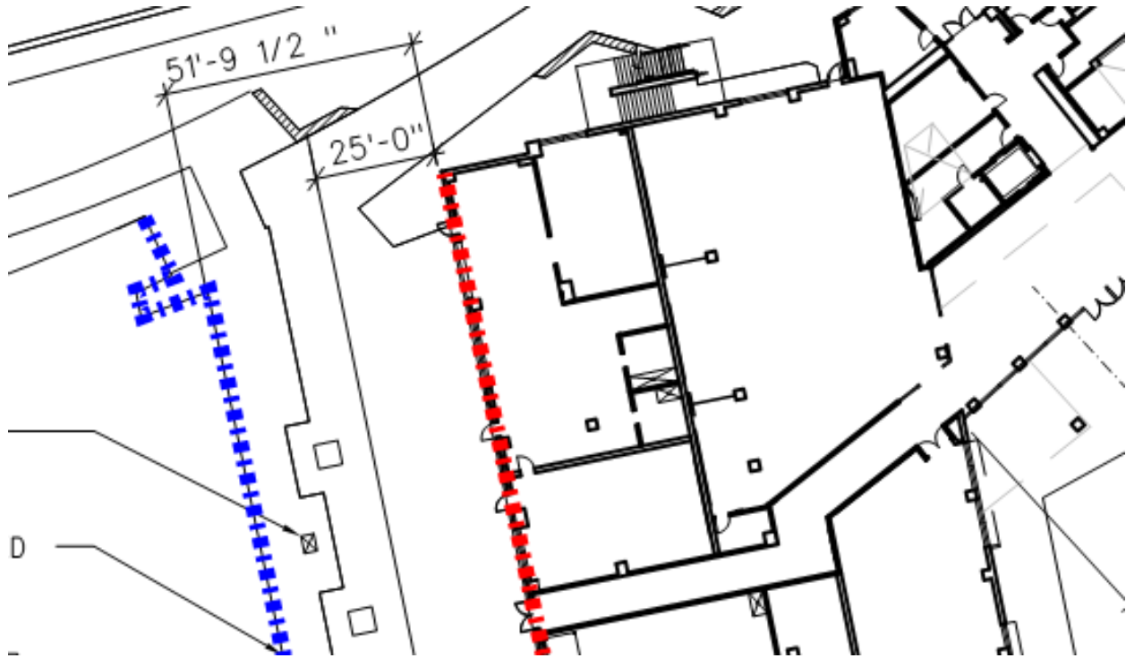
Figure 18. Fire separation distance between Engineering IV and Engineering III. The imaginary property line is located at the approximate midpoint between the two buildings, resulting in 25-feet of FSD for each building. The exterior wall of Engineering III (left) is a 3-hour rated CMU wall (shown in blue), while the exterior wall of Engineering IV (right) is 1-hour rated (shown in red).
