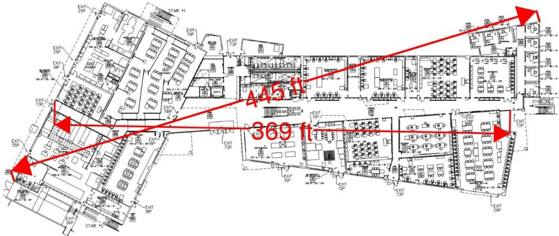
Figure 3. Exit separation distance for the first floor. The two farthest exits serving the main corridor are 369-feet apart, greater than one-third the maximum separation distance of 445-feet.
