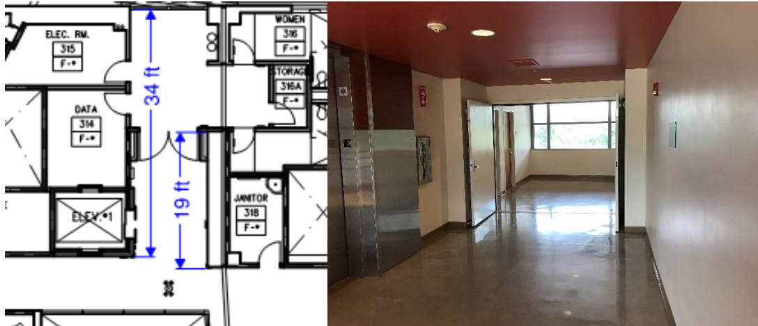
Figure 8. The 20-foot dead-end limit required for Group A occupancies is not exceeded in the corridor due to the addition of magnetic closing doors.
