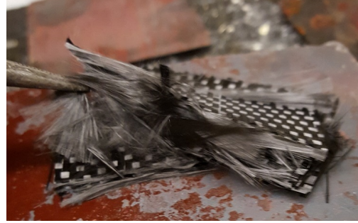
(b) Individual fibers can be seen in the specimen after burning epoxy
