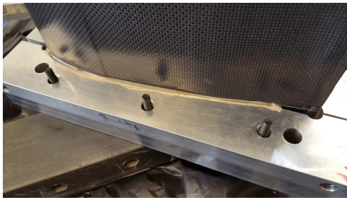
(a) Cured epoxy used to fill boundary condition void
