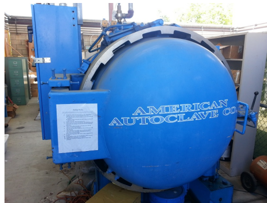
(b) Autoclave to make composite parts with complex geometries
