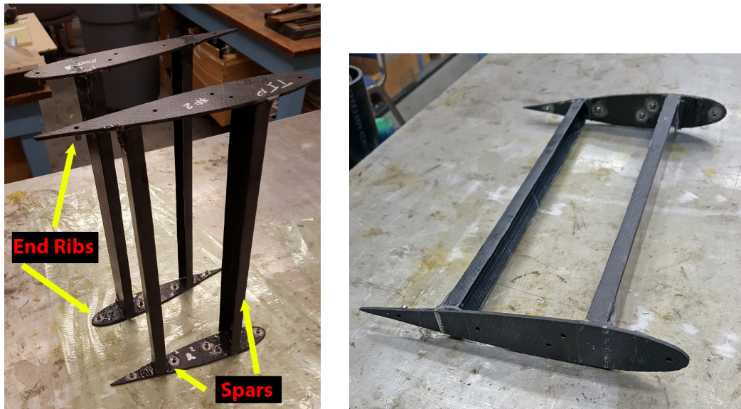
(a) Second rib is placed on spars and bonded (b) Finished internal structure of wing model
