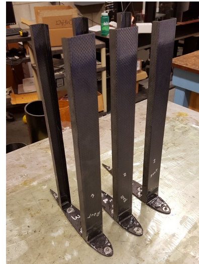
(b) Leading and trailing edge spars bonded on to rib
