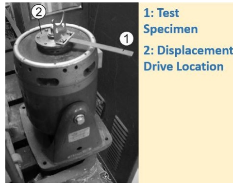
Figure 1.9: Shaker used to apply a resonance on a test sample so that the modulus could be calculated [7]
