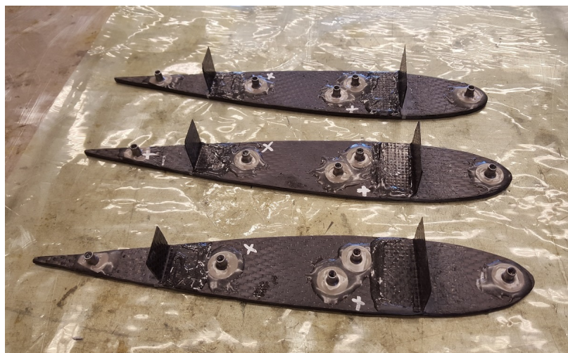
Figure 3.20: Inner brackets bonded to provide pressure when bonding spars
