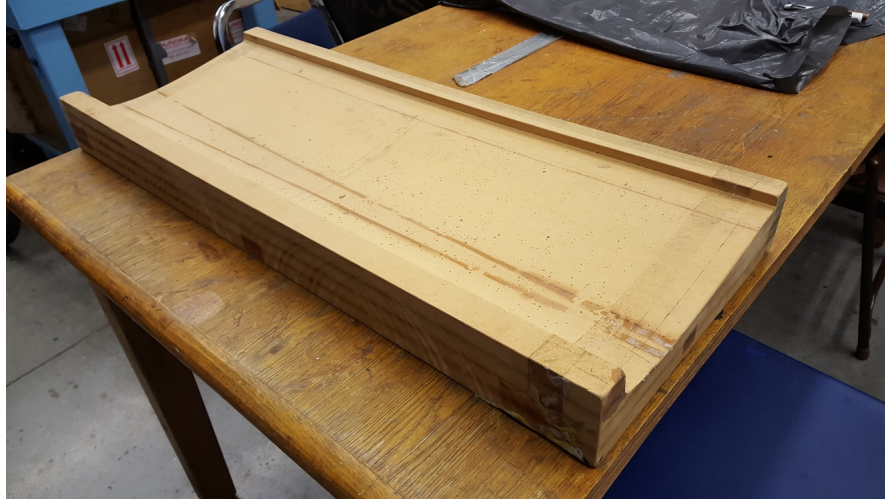
Figure 3.5: Finished female mold ready to be used for skin layup
