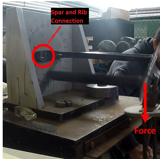
Figure 2.10: Picture of prototype wing failure at the root and spar connection
