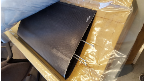
(a) Female skin mold used to hold assembly while curing
