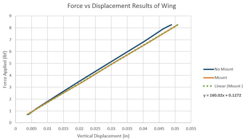
Figure 5.13: Comparison of the force and displacement study with and without the front mount
