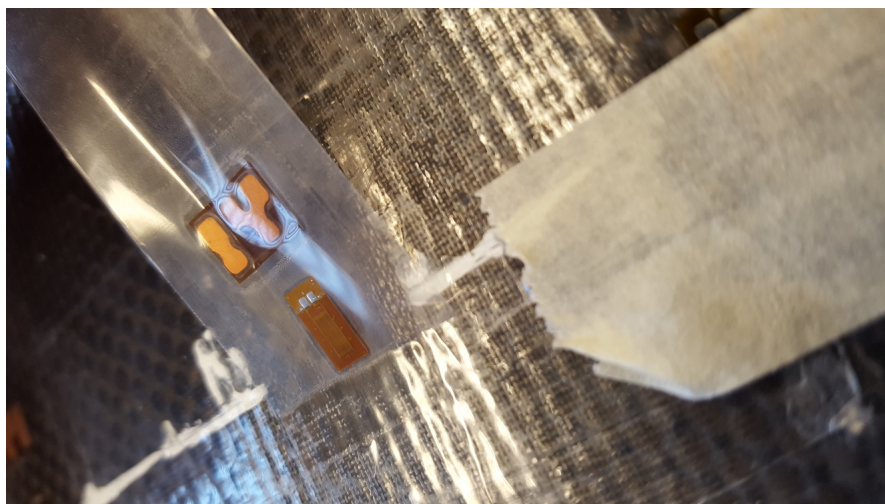
Figure 3.27: Uni-directional strain gage and terminal ready to be applied to bond surface
