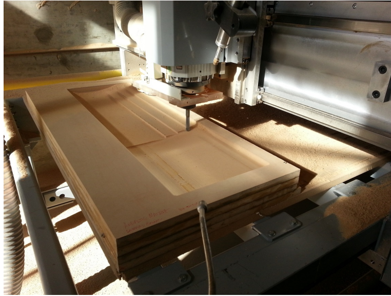
Figure 3.4: Machining of female wing skin mold in progress
