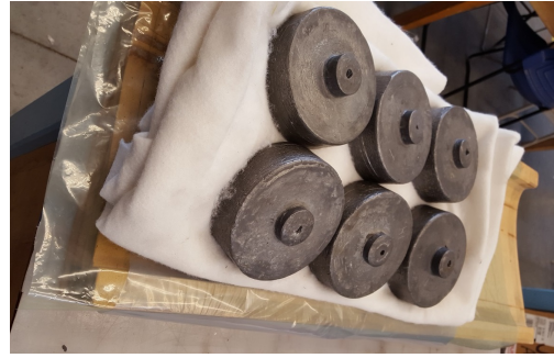
(b) Weights used to apply pressure for bonding
