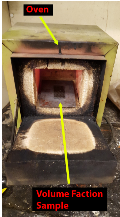
Figure 4.17: Oven used to burn the epoxy out of the carbon sample for volume fraction calculations
