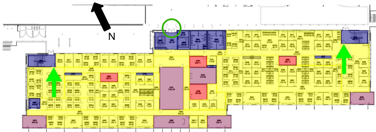
Figure 5: First Floor Exits and Occupancy Use
