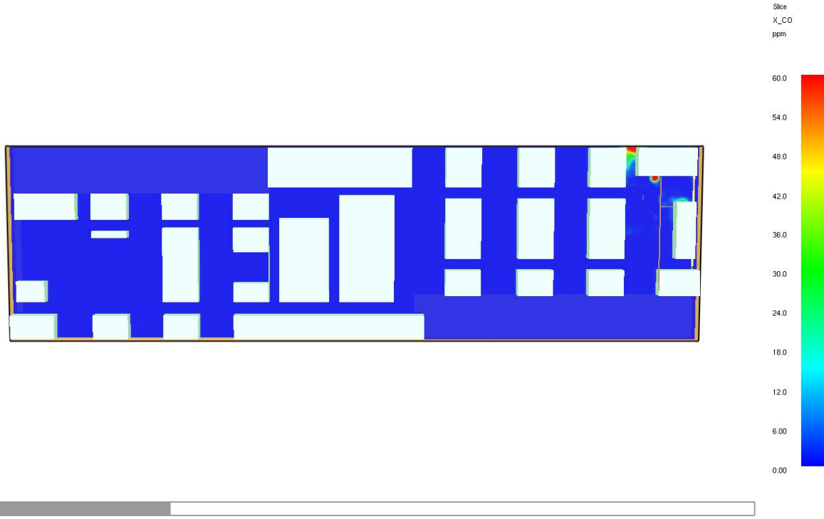
Figure 49: FDS Carbon Monoxide Level at 165 Seconds
