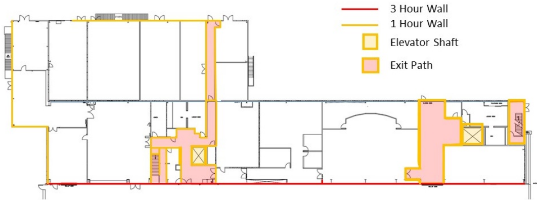
Figure 3-2: Ground Floor Office Area Fire Resistance Requirements
