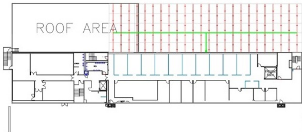
Figure 6-17: East Overhang deluge Sprinkler system layout
