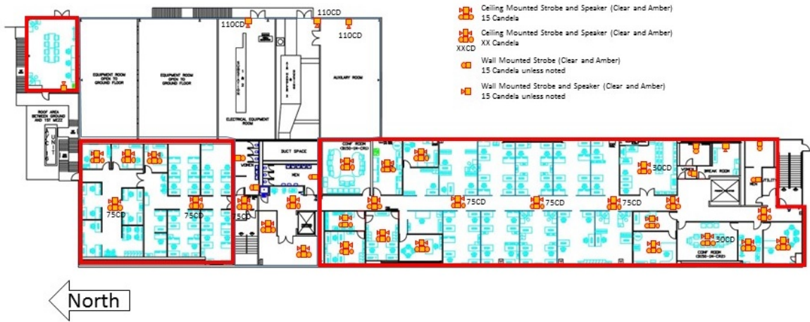
Figure 5-15: Notification Device Locations (2 nd Floor)
