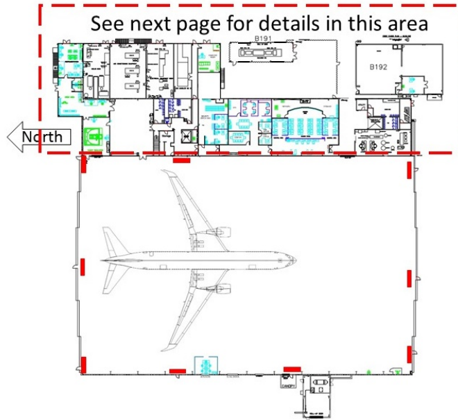
Figure 4-9: Exit Sign locations in Hangar Bay
