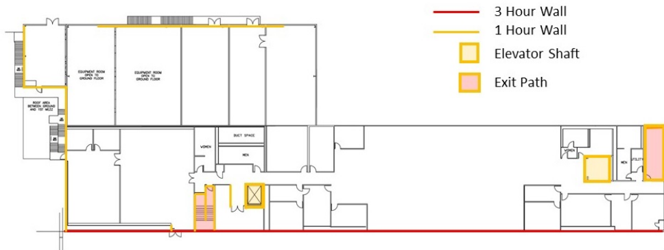
Figure 3-3: Ground Floor Office Area Fire Resistance Requirements
