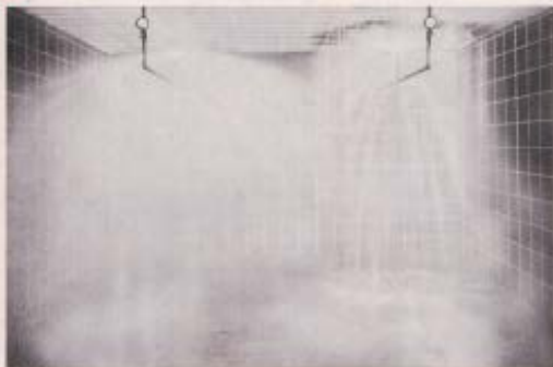
Note superior distribution and breakup of pattern between SPRAY Sprinkler, left and conventional sprinkler, right. Heavy water droplets from regular sprinkler form distinct pattern on floor.
