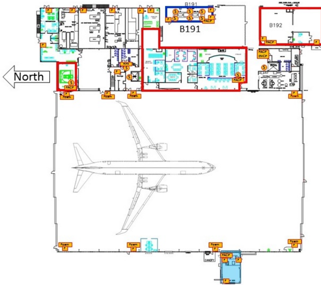
Figure 5-5: Pull Station and Detector Locations (Ground Floor)
