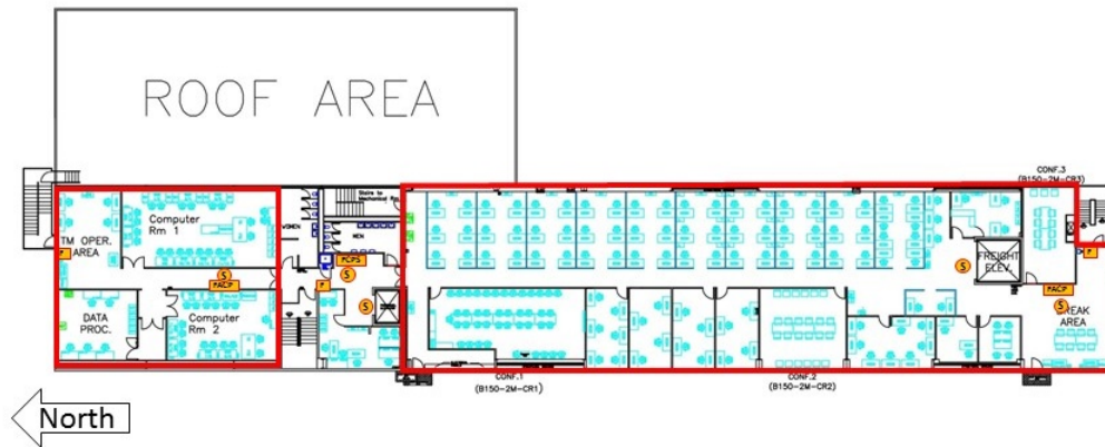
Figure 5-7: Pull Station and Smoke Detector Locations (3 rd Floor)
