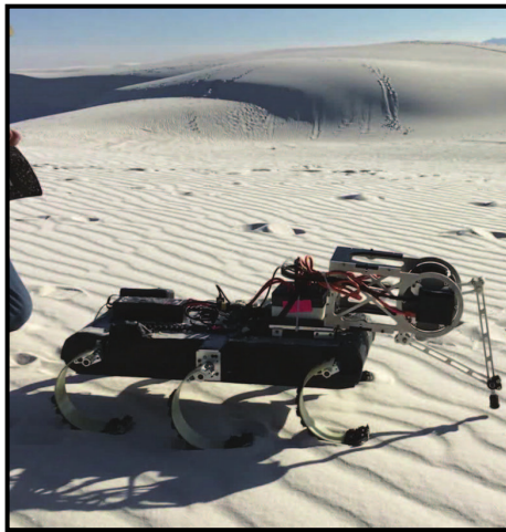
Figure 3.2: An example of the recently developed RHex robotic platform deployed in the field in White Sands, NM. The robot is outfitted with a probe assembly mounted near the front of the body. The probe uses force feedback from two motors to obtain force and position output that can be used to perform various mechanical tests of the sand surface.
