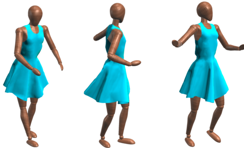
Figure 5.5: Character clothing with continuous collision detection, including both cloth-body and cloth-cloth collisions.
