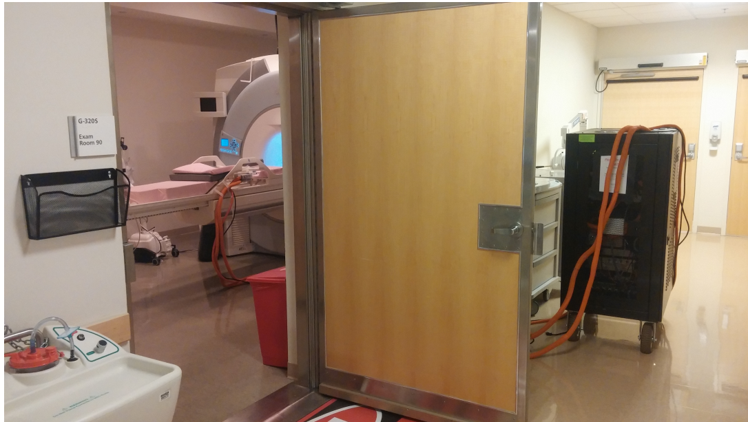
Figure 6.6: DOT-MRI System in MR Suite. When in use, the DOT instrument rack is brought to the control room of the MR suite at the Hospital of the University of Pennsylvania. The fiber bundles then pass through the waveguide and are incorporated into the clinical breast biopsy RF coil, on which the subject can lie in a prone position to be simultaneously imaged by MRI and DOT
