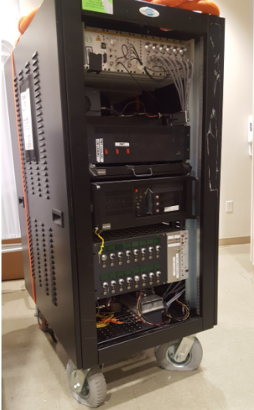
Figure 6.2: DOT-MRI Instrument Rack. The optical and electronic components of the DOT-MRI instrument are housed within an instrument rack on pneumatic wheels for easy transport to and from the MR suite. This rack contains all laser sources, the pulsed laser diode driver, all optical switches, the CW detection fiber imaging plate and CCD, PMTs and PMT control-units for TD detection, and TCSPC control instrumentation.
