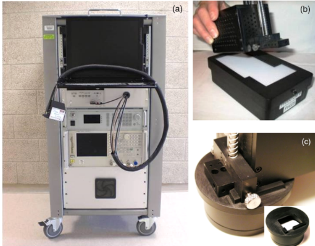
Figure 3.3: DOSI Instrumentation and Hand-piece. This figure comes from [166]. A) DOSI Opto-Electronics Rack. This instrument cart contains the white-light source, laser diodes, spectrometer, frequency analyzer, and instrument control computer for the DOSI system. Several systems similar to this collected all of the DOSI data in Chapters 3, 4, and 5. Note that the instrument is portable and can be wheeled to the patient’s bedside. B) DOSI Hand-piece and Calibration Phantom. The DOSI hand-piece contains an APD for frequency-domain detection and optical fibers coupled to the optical components on the instrument rack. A calibration phantom, placed inside a case for easy alignment with the hand-piece, is also shown. C) DOSI Hand-piece and Reflectance Standard. The DOSI hand-piece is shown in contact with the broadband reflectance standard. Note that the fiber-coupling apparatus can easily be moved to three different positions, using the silver spring-loaded hand screws seen here, to provide multiple source-detector separations.
