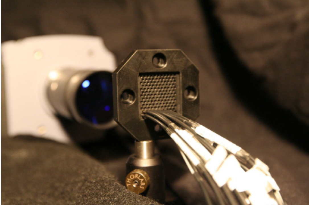
Figure 6.3: Detection Fiber Plate and CCD. CW detection fibers and the CW reference channel are mounted onto a plate which is then imaged onto a CCD. The spot on the CCD from each fiber tip can then be used as an individual detector. Note that this is a photograph of the plate in the early stages of construction [52], prior to completion of the system; the final version contains considerably more fibers.
