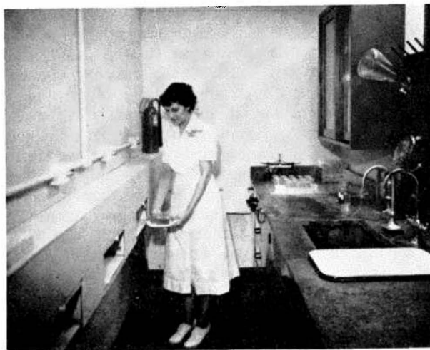
FIG. 2. The preparation area of the taste panel room at the Northern Regional Research Laboratory. The attendant is passing samples of oil in a heated aluminum block to the taste panel member on the opposite side of the partition.
