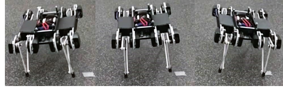
Figure 20. Snapshots of pacing in place (taken roughly at left stance, aerial, right stance) from the experiment in Fig. 23(center, right).
