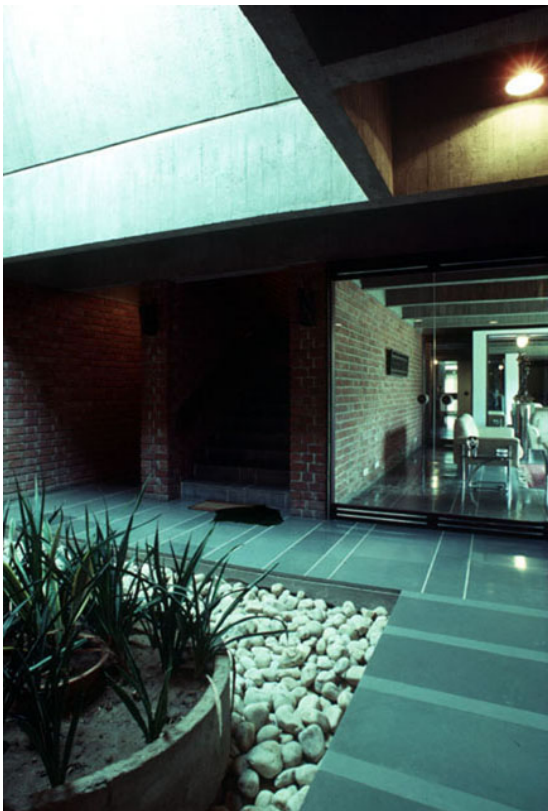
Fig. 46: "Tube House" concept of using a roof opening to illuminate and ventilate interior spaces (Source: Hassan Uddin Khan)
