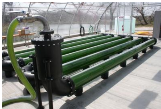
Figure 4.4: Transparent horizontal tubes are used for growing algae, often outdoors, to take advantage of sunlight (Climate Tech Wiki).
