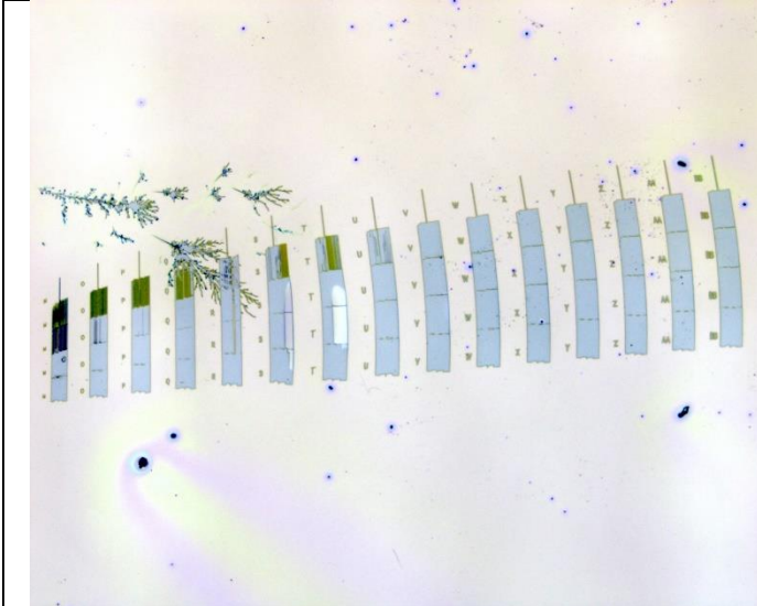
Figure 4a. Without DisCharge, charge accumulation leads to poor shape fidelity of the tower patterns.
