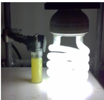
Figure 2.10: Photoredox cross-coupling reaction set-up (0.5 mmol scale)
