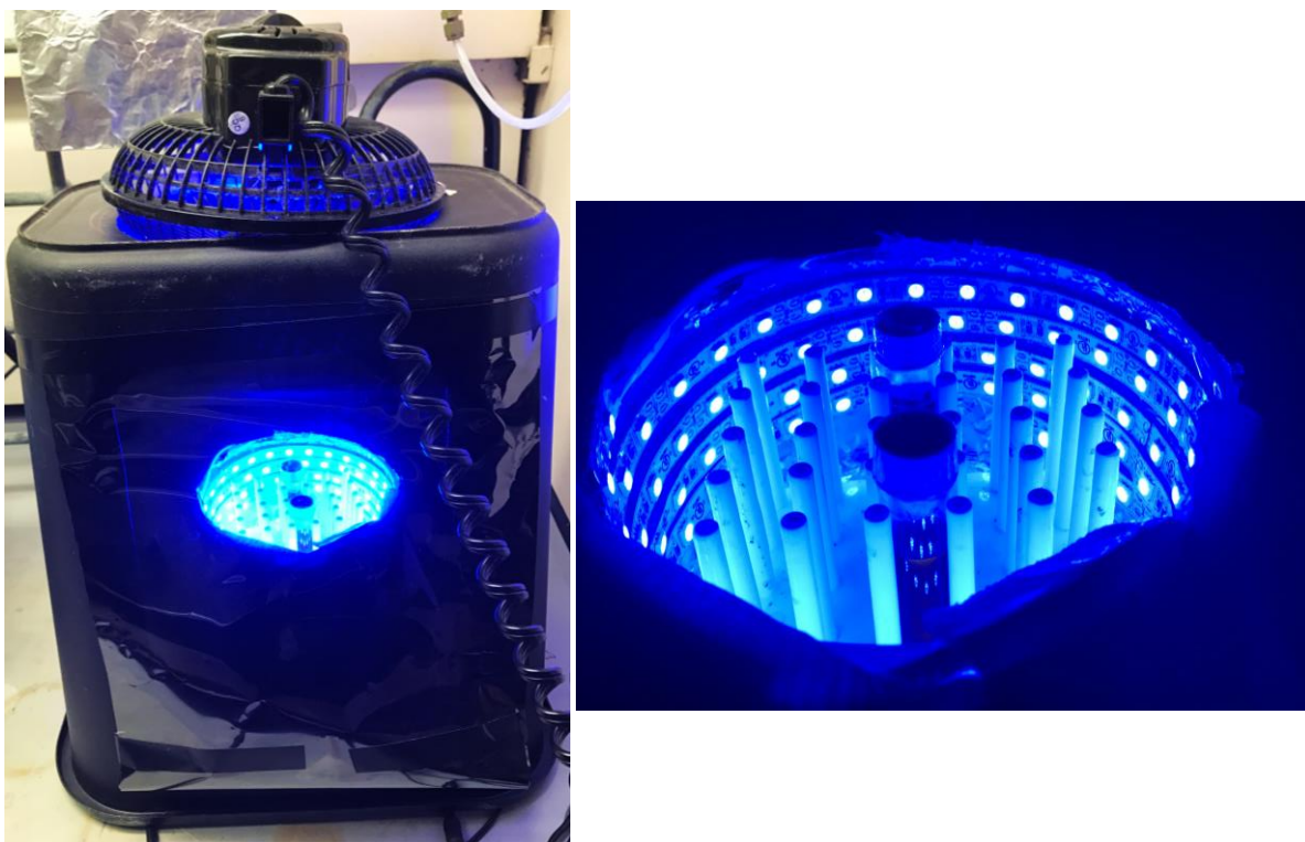
Figure 6.12. Procedure B photoredox cross-coupling reaction set-up (0.50 mmol scale)
