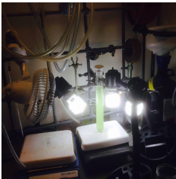
Figure 4.8. Gram scale photoredox cross-coupling reaction set-up (4.65 mmol)
