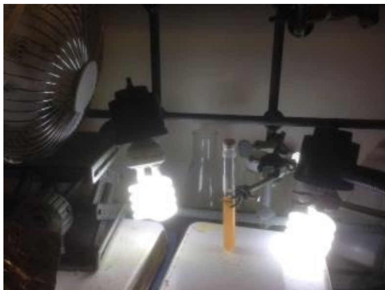
Figure 4.7. Photoredox cross-coupling reaction set-up (0.5 mmol scale)
