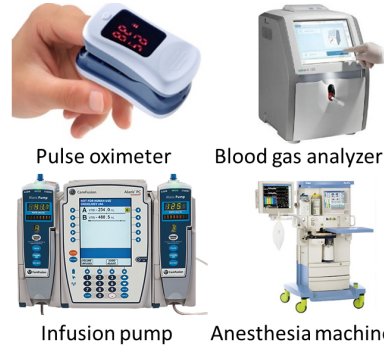
(b) Typical medical devices used in an operating room: a pulse oximeter [4], a blood gas analyzer [3], an infusion pump [1] and an anesthesia machine [5].
