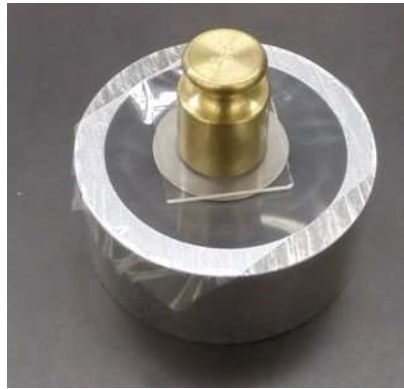
Figure 5-1: Image of a specimen during the preparation process. The 200 g weight was placed on top of the washer while the cyanoacrylate was curing. The PET film was mounted on a two-inch ring in this image.
