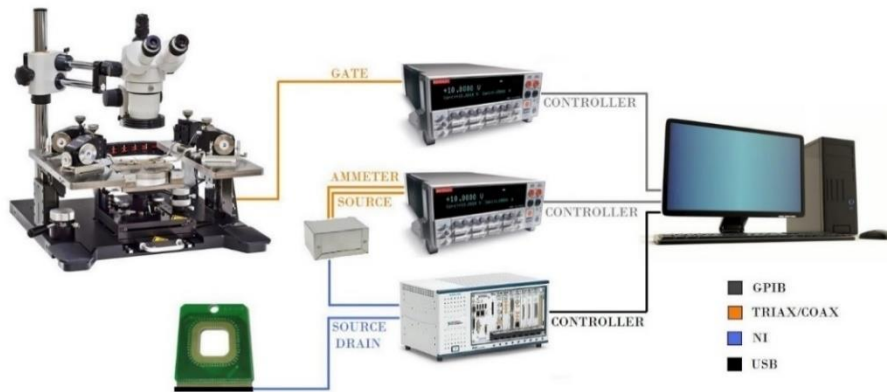
Figure 3.2: Parallel electrical characterization setup. Two Keithley source meters, a probe card, a switching matrix, the probe station, and a controller computer are shown.
