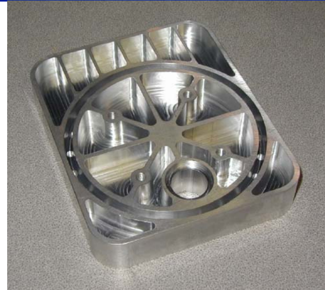
Exhibit CNC. Aluminum part flexibly produced by a CNC milling machine. A web-based design program can be used to create instructions for the milling machine. Source: emachineshop.com.
