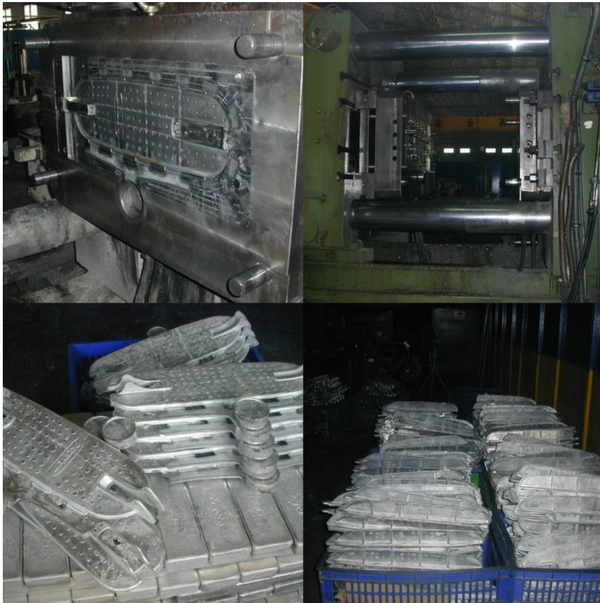
Exhibit PRODUCTION. Production of the Mg deck requires a die (or mold) as shown in the upper two panels. The raw castings as they come from the die are shown in the lower two panels. The lower right panel shows a production batch of about 500 pieces.
