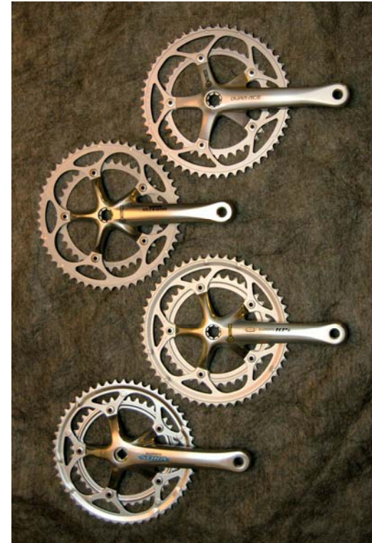
Exhibit CRANKS. Shimano bicycle cranks are available in several different quality levels for a given size and application type. These four artifacts are all 170mm 53/39-tooth cranks sold by Shimano at prices from $60 (bottom) to $350 (top). This is an example of quality variety.
