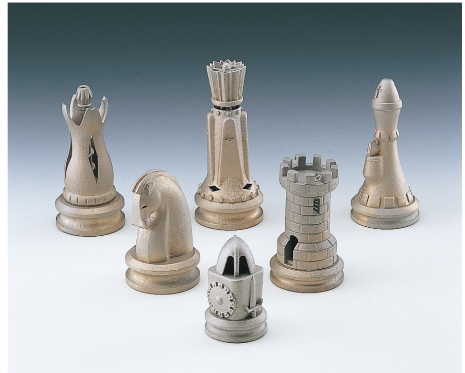
Exhibit SLS: Chess pieces fabricated using the Selective Laser Sintering (SLS) process, a rapid prototyping technology. Source: http://www.kinzoku.co.jp/image/zoukei_p3_b.jpg
