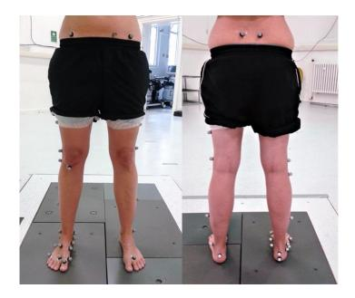
Figure 3.2: Marker Placement for the Conventional Lower Limb Model
