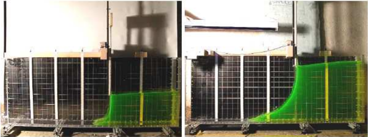
Figure 5.24. Free surface profile and upstream wave at the instant of complete dam gate removal. H = 300 mm (left), H = 600 mm (right).
