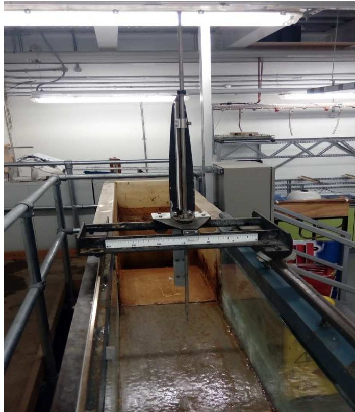
Figure 4.4. Point gauge (manually operated) for measuring scour profile.
