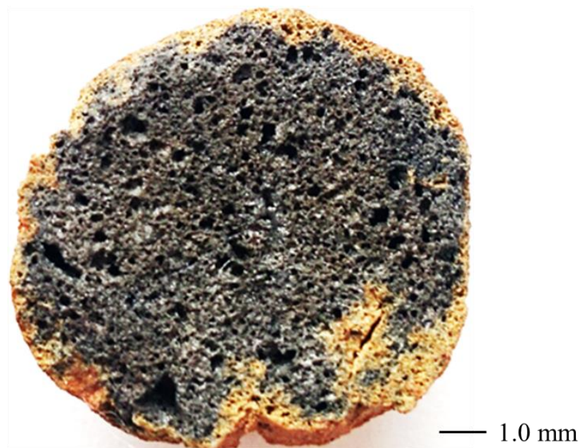
Figure 2.9 Ideal pore structure shown for an individual clay LWA pellet (Ayati et al., 2018).
