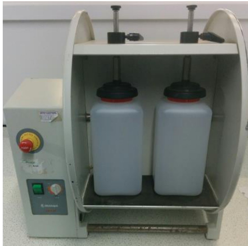
Figure 3.4 End-to-end rotary tumbler used for leaching test.
