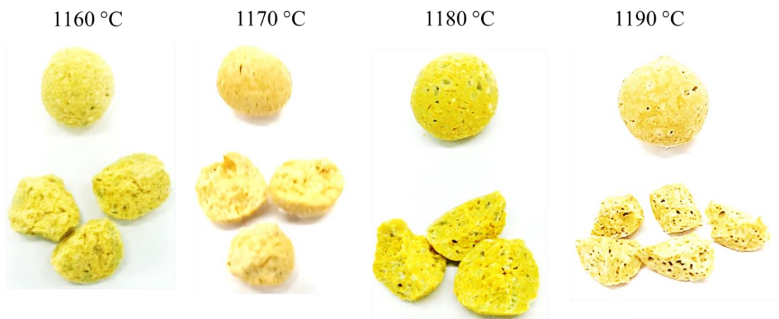
Figure 7.2 Appearance of the surface and internal structure of (a) SDC-LWA, (b) CDC-LWA and (c) EDC-LWA with 40 wt.% added glass.
