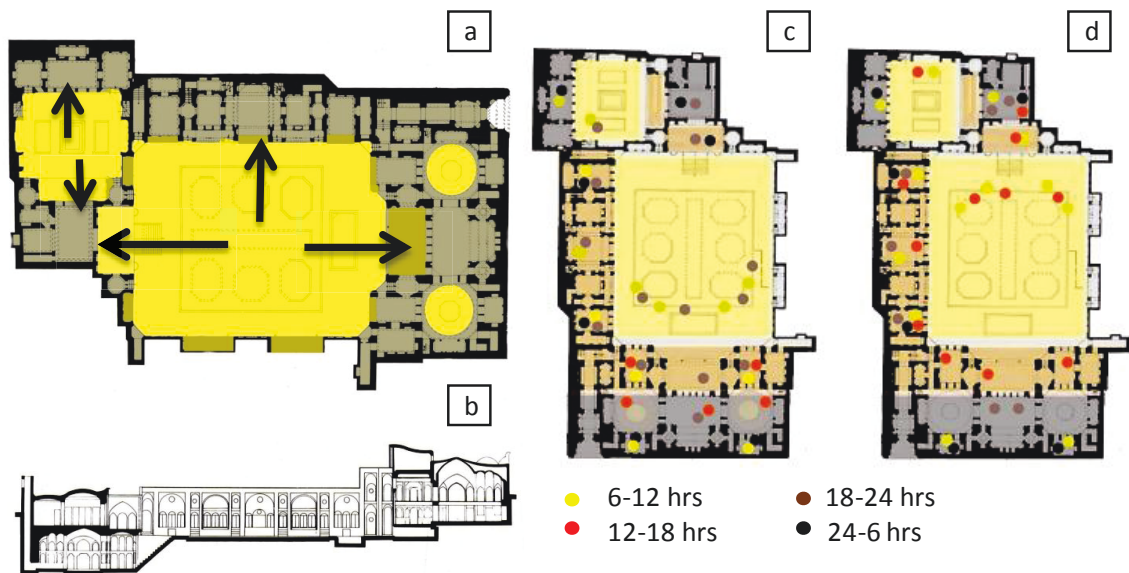
Figure 4. Tabatabaei benchmark house - [a] direction of daylight from courtyards to interior spaces – plan view; [b] Elevation view; seasonal spatial distribution of occupants over the course of day [c] Summer season [d] Winter season (Farokhyar, 2013 with modifications)
