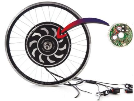
Fig. 4. The wheel hub motor which includes a built in driver [8].
