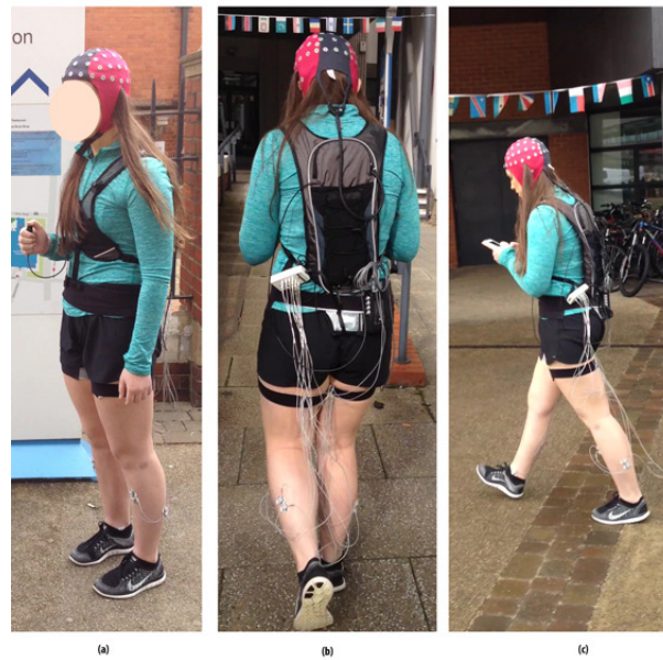
Fig. 1: A typical participant wearing high-density 64 channel Waveguard Cap and other measurement sensors. (a) Front view , b) Back view and (c) Walking & texting during experiment.
