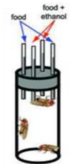
Figure 2.6: CAFE vial highlighting the capillary containing liquid foods. Image used with permission from Devineni and Heberlein (2009).
