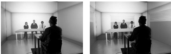
Fig. 1. The enclosed and the room with openings. Due to the stereoscopic projection the participant will experience a clear 3D environment, in which the floor continuous unhindered to the horizon through the openings.
