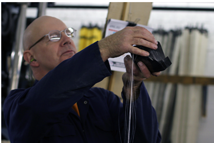
FIGURE 9. ‘Shining’ the carriages to look for irregularities.
