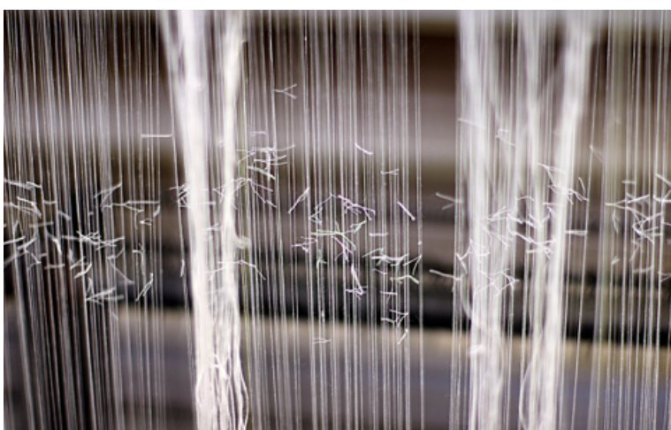
FIGURE 3. Knots linking old and new threads.
