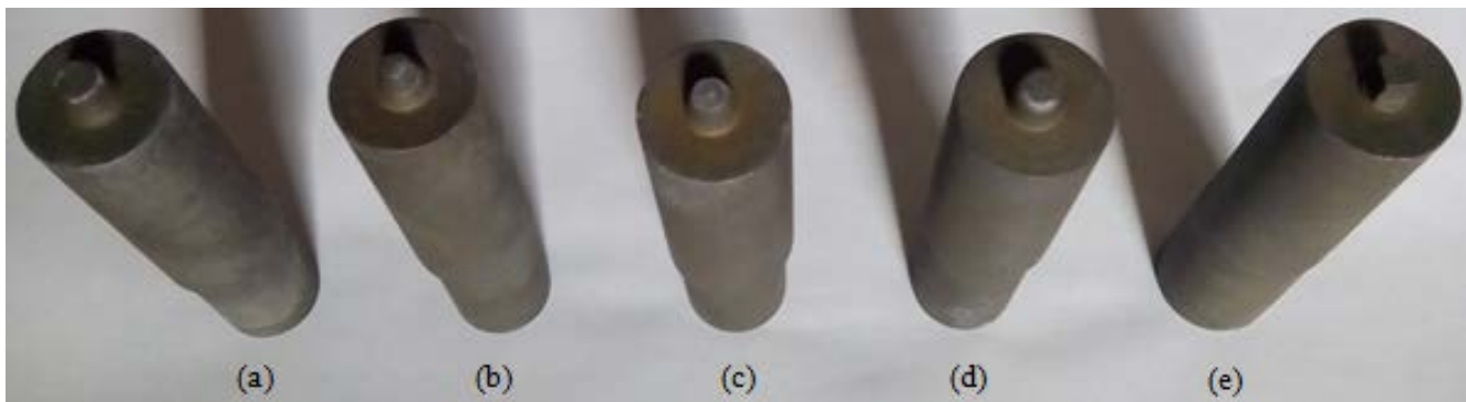
Figure 1. Manufactured tools (a) cylindrical threaded (b) tapered threaded (c) simple tapered (d) simple cylindrical (e) simple square
