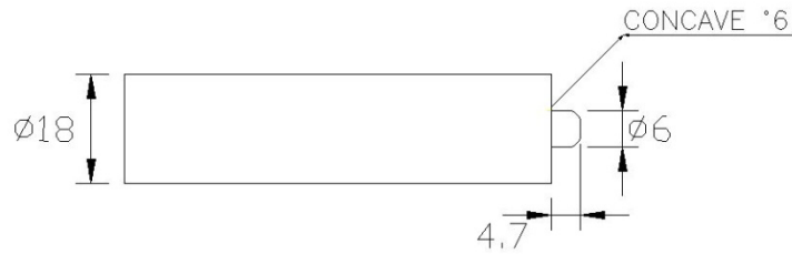
Figure 2. Conceptual diagram of simple cylindrical tool
