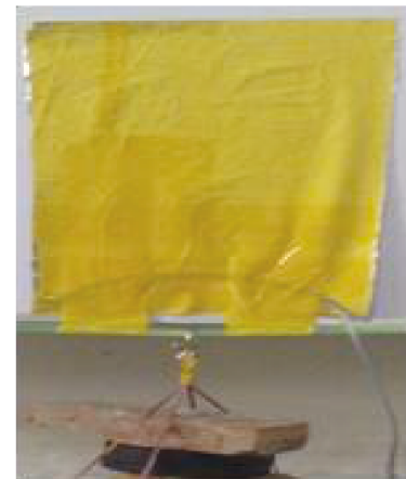
Figure 4 Unipolar electroadhesion pad for robot
