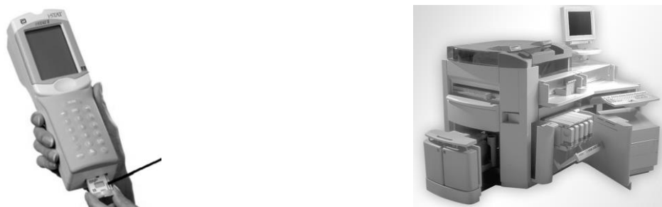
Figure 7.3 Left: Portable (handheld) blood analyzer i-STAT System which provides real-time, lab-quality results in minutes (Rios et. al., 2012:7). Right: Full size, floor standing blood analyser (Nottingham Spirk, 2012).
