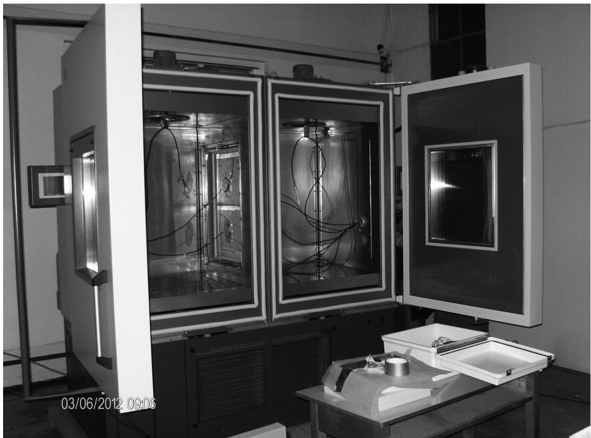
Figure 6.35: The insulation materials between the hot and cold chamber with all the sensors installed.
