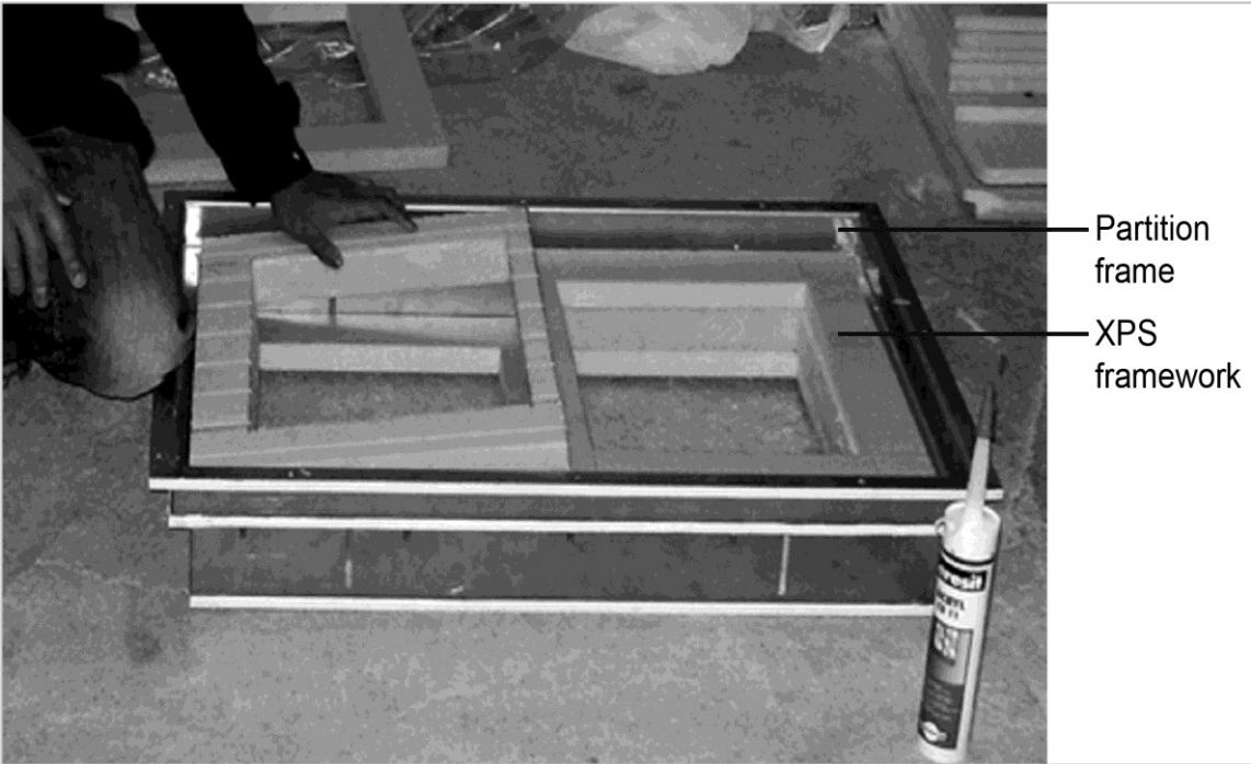
Figure 6.33: The XPS framework and the partition frame.
