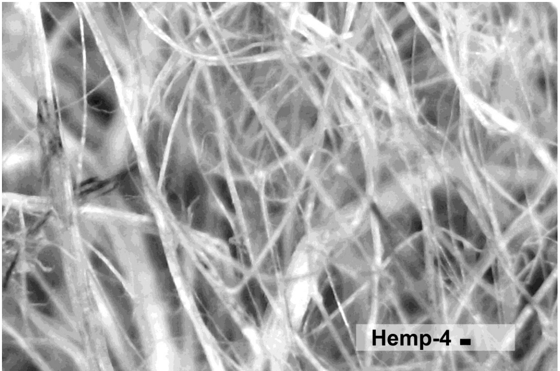
Figure 4.14: Microscopic image of the sample of the hemp-4 insulation. Scale bar: 100 \mu\text{m} .
