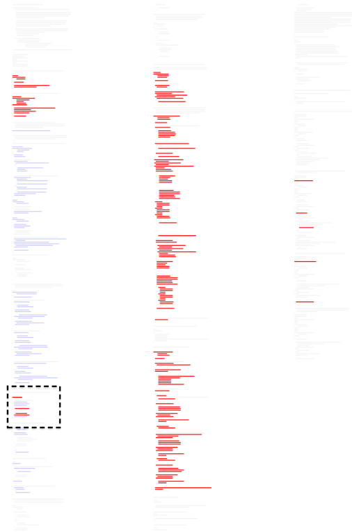
Figure 7: File View for the file util.c of Program bc . Each line of pixels correspond to one source code line. Blue (medium gray in black & white) represents lines with vertices belonging to the 2^{nd} largest cluster and red (dark gray) represents lines with vertices belonging to the largest cluster. The rectangle marks function init_gen , part of both clusters.
