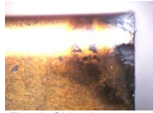
Fig 2b-Side view (flank) modified tip after 30 passes
