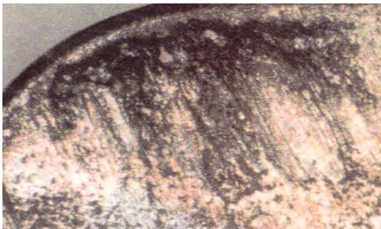
Figure 3.8: SEM image showing marks left by chips sliding over tool rake face
