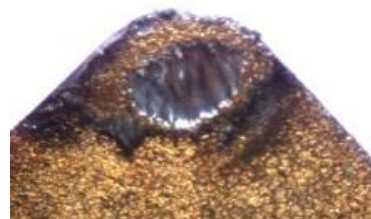
Fig 2b- Rake face modified tip after 30 passes
