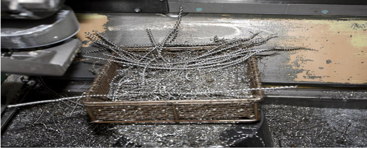
Figure 4.5: showing long shiny Swarfs in a Tray in the machining centre compartment.
