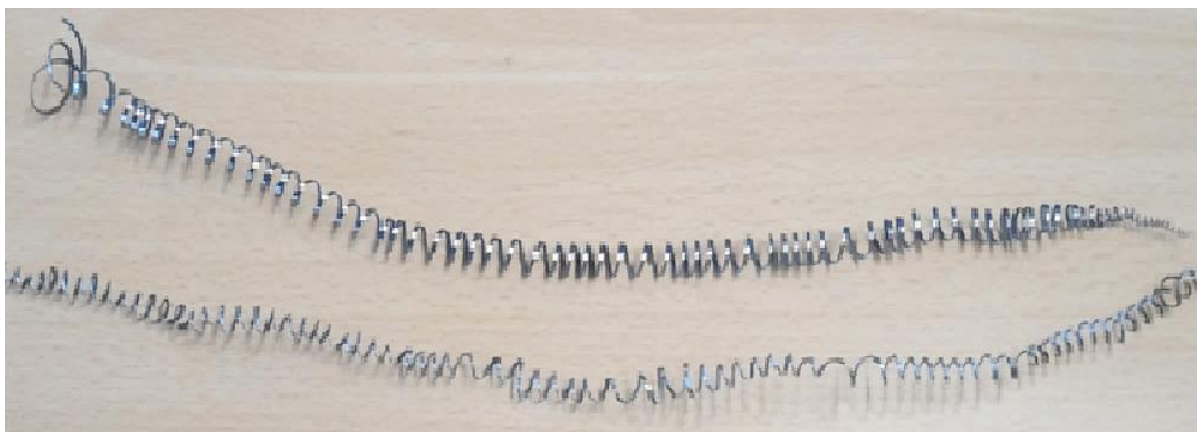
Figure 4.2: Long Shiny Swarfs Generated by EDMed Modified Tool. Chip thickness was 1.43 mm
