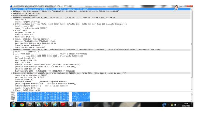
Figure 71: Using 6to4 techniques by encapsulating IPv6 in IPv4 header
