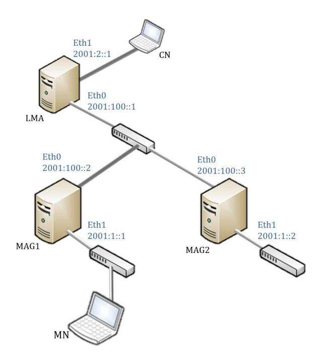
Figure 43: The topology of PMIPv6 test bed
