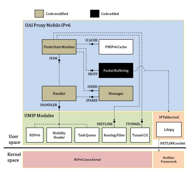
Figure 34: OAI PMIPv6 including buffering module
