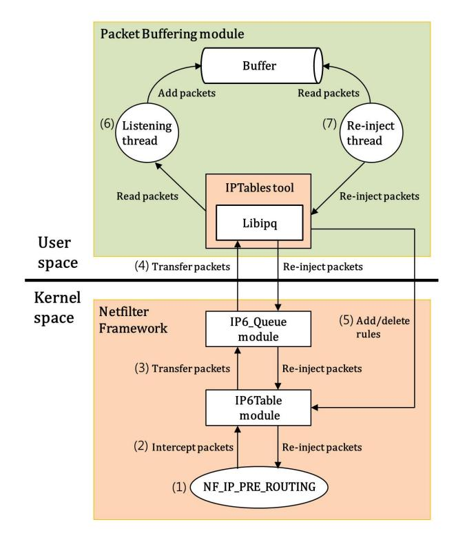
Figure 35: Operation of Packet Buffering Module
