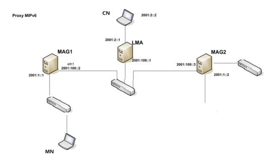
Figure 73: The real testbed of Proxy MIPv6 representation
