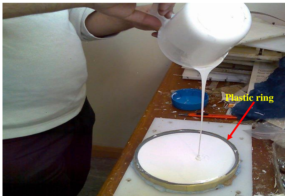
Fig 5.14: Mould preparation by using clamps to hold ring.
