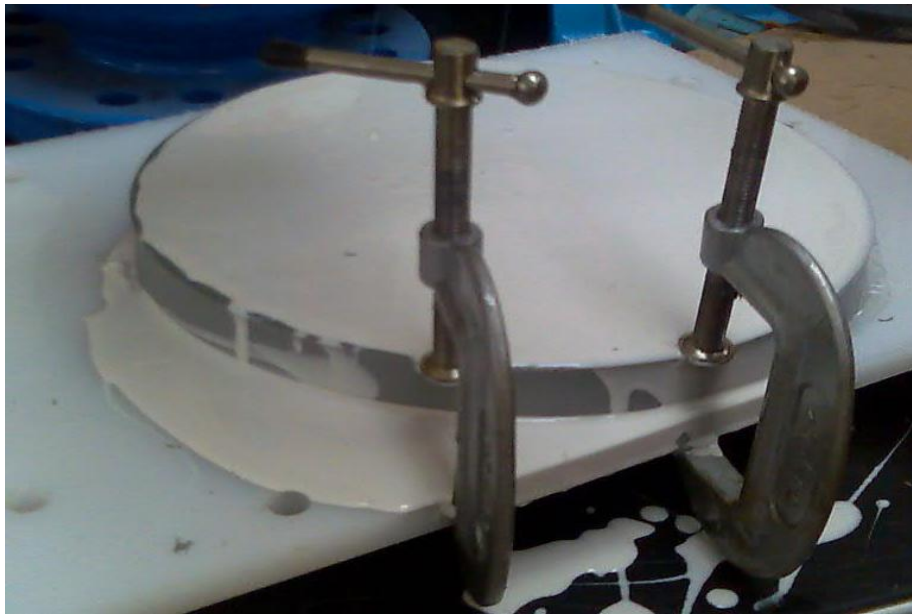
Fig 5.15: Another mould Preparation by using catalyst and curing agent
