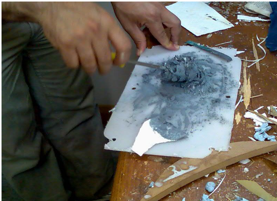
Fig 5.17: Mixing of silicon carbide with araldite epoxy resin
