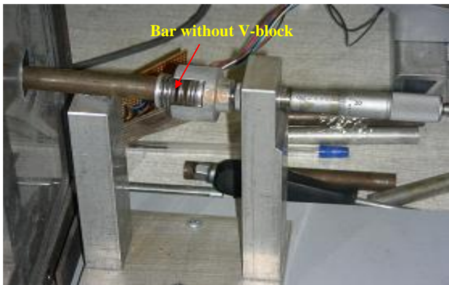
Fig 5.10: Constructed assembly holding bar without V- block
