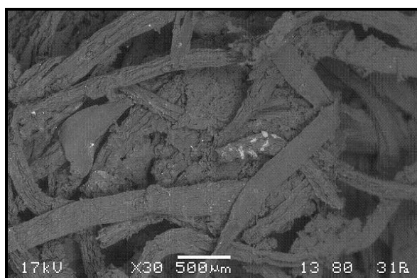
Figure 7: SEM photo for Fen peat (Holme Post site)
