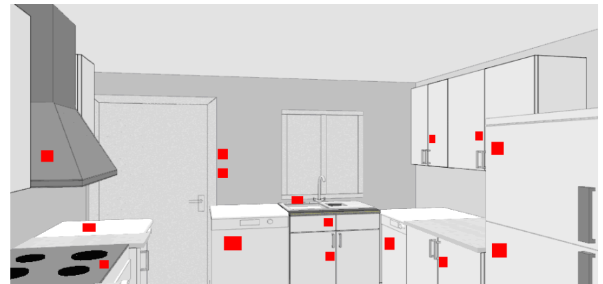
Figure 4 - The kitchen showing all the locations of the passive transponders
